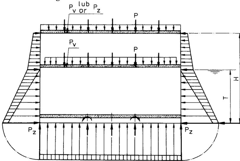
Fig. 2.3.1 Load condition LC3
