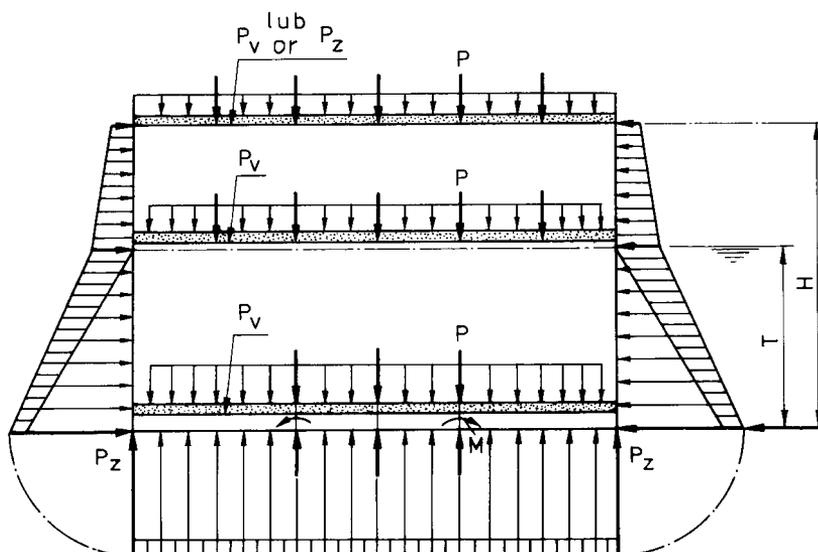
Fig. 2.1.1 Load condition LC1
