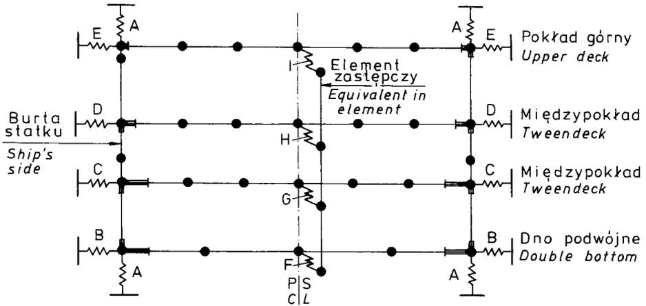
Fig. 3.2.1-2 Transverse web frame between pillars
