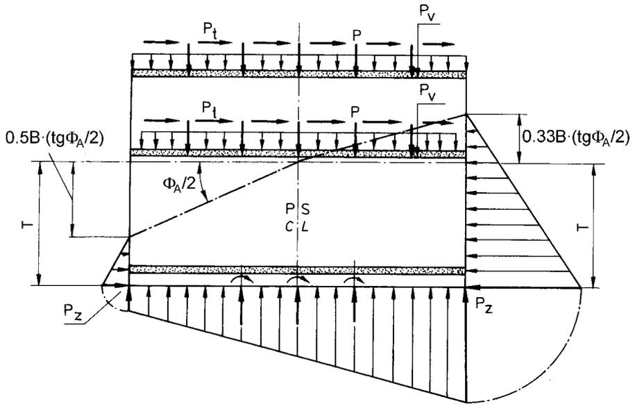
Fig. 2.4.1 Load condition LC4
