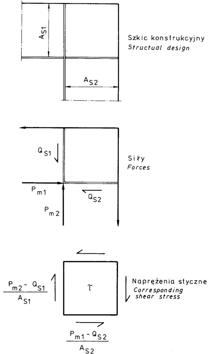
Fig. 4.2.1 Stress analysis of cross joint
