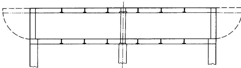
b) Grillage model (upper deck), including ship's sides unfolded
