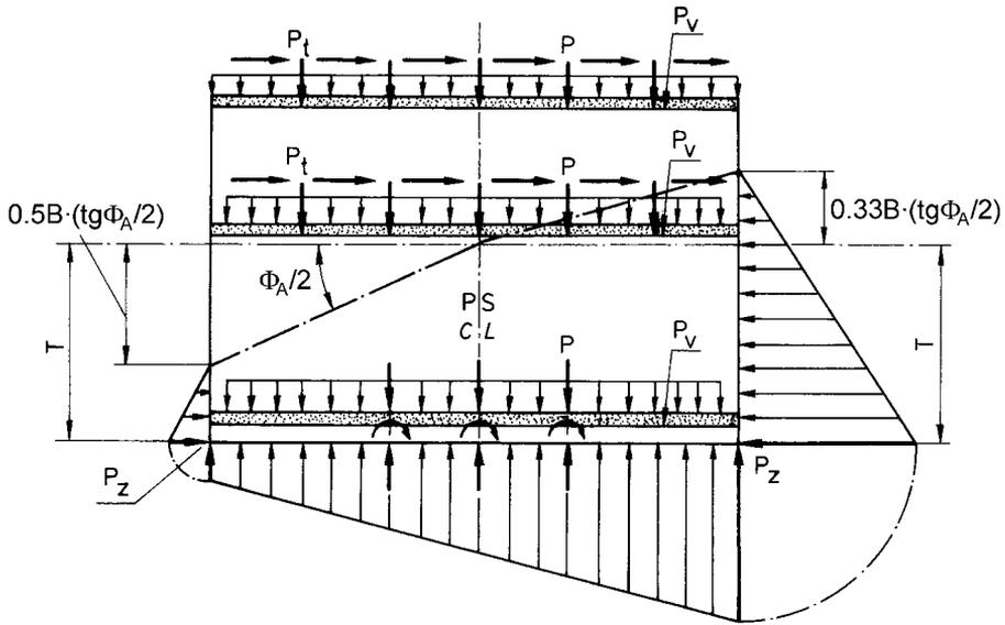
Fig. 2.2.1 Load condition LC2
