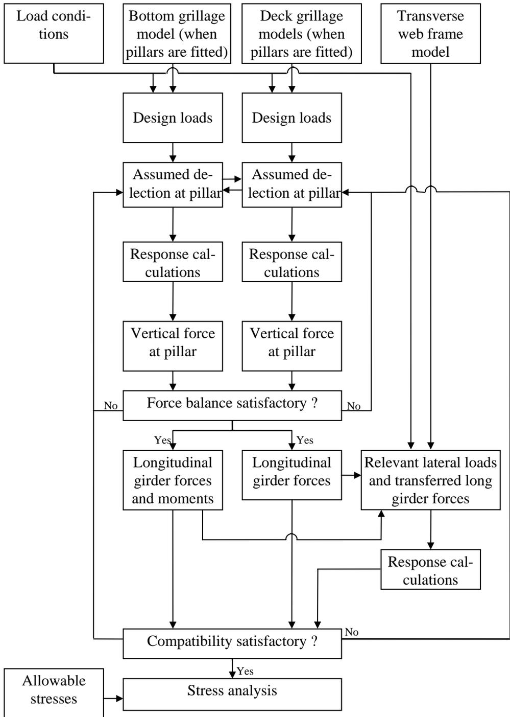
Fig. 1.2.1 Strength analysis procedure of roll on/ roll off ship
